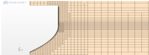
Fig. 4: Transverse intersection of the mesh around the midship section of the Wigley hull, showing local refinement near the free-surface.
