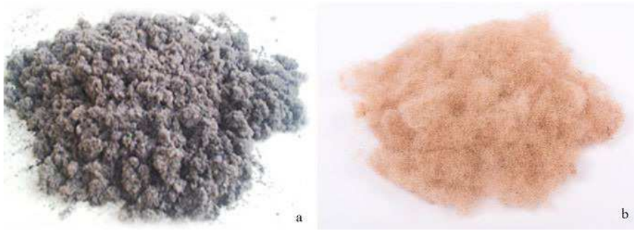
Fig. 1. (a) Waste fibre before the cleaning process; (b) cleaned fibre for use in concrete (RTPF)
