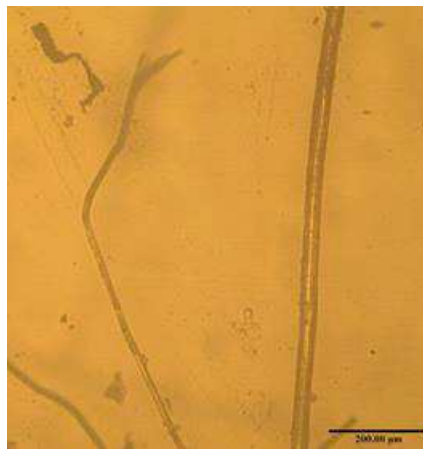
Fig. 2. RTPF enlarged 100 times using an optical microscope
