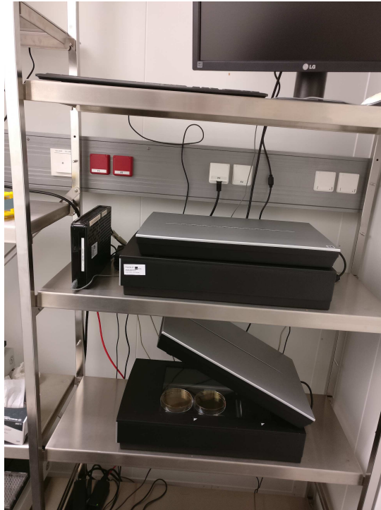
Appendix figure 3. Image of the scanner system. Photograph of the scanner system used for time-lapse imaging of phage spread in spatially structured bacterial populations. Three scanners (Epson Perfection V600 Photo Scanner) simultaneously scanned 12 plates in total every 20 minutes in 30°C for 48 hours per experiment.
