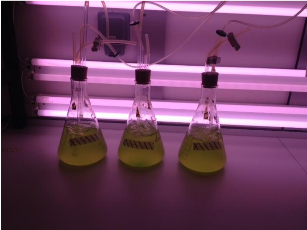
Figure 2.19. C. vulgaris being cultured in BBM under aeration and exposed to UV light.
