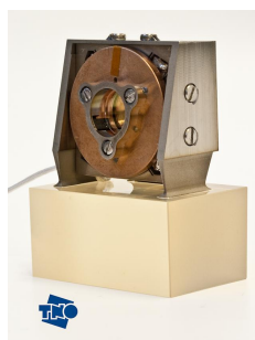
Fig. 6. FSUA Breadboard on a Zerodur test carrier.
