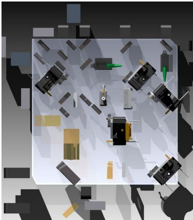
Fig. 5. CAD drawing of the telescope simulator with a mirror and a quarter-wave plate for the commissioning of the telescope simulator.
