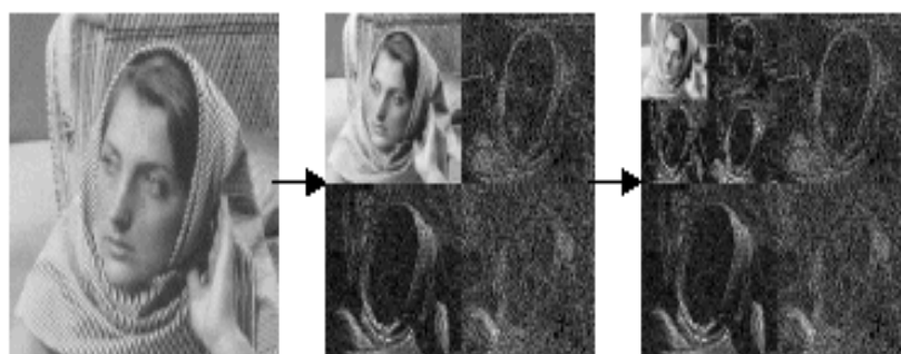
Figure 25: Example of dyadic decomposition [56].
