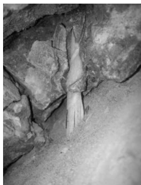
Figure 13 GFRP DE bar in specimen G150 \Delta (1.6% strain)
