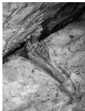
Figure 14 CFRP DE bar in specimen C150 \Delta (1.5% strain)
