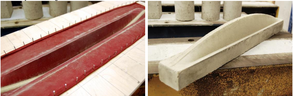
Fig. 3 Formwork for (left) and finished (right) beam K2
