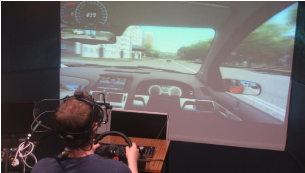
Figure 1. The basic experimental set up. Participants wore an eye tracker and were seated in front of a calibration screen and main projection screen.
