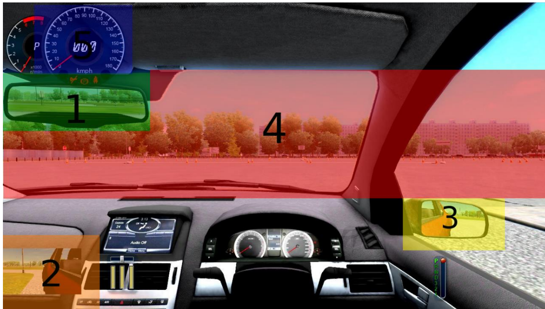
Figure 5. Illustration of each area of interest. 1) Rear-view mirror (16 deg x 5 deg); 2), Passenger-side mirror (12 deg x 5 deg); 3), Driver-side mirror (19 deg x 7 deg); 4) Roadway (58 deg x 27 deg at maximum length and height), 5) Speedometer (12 deg x 9 deg).
