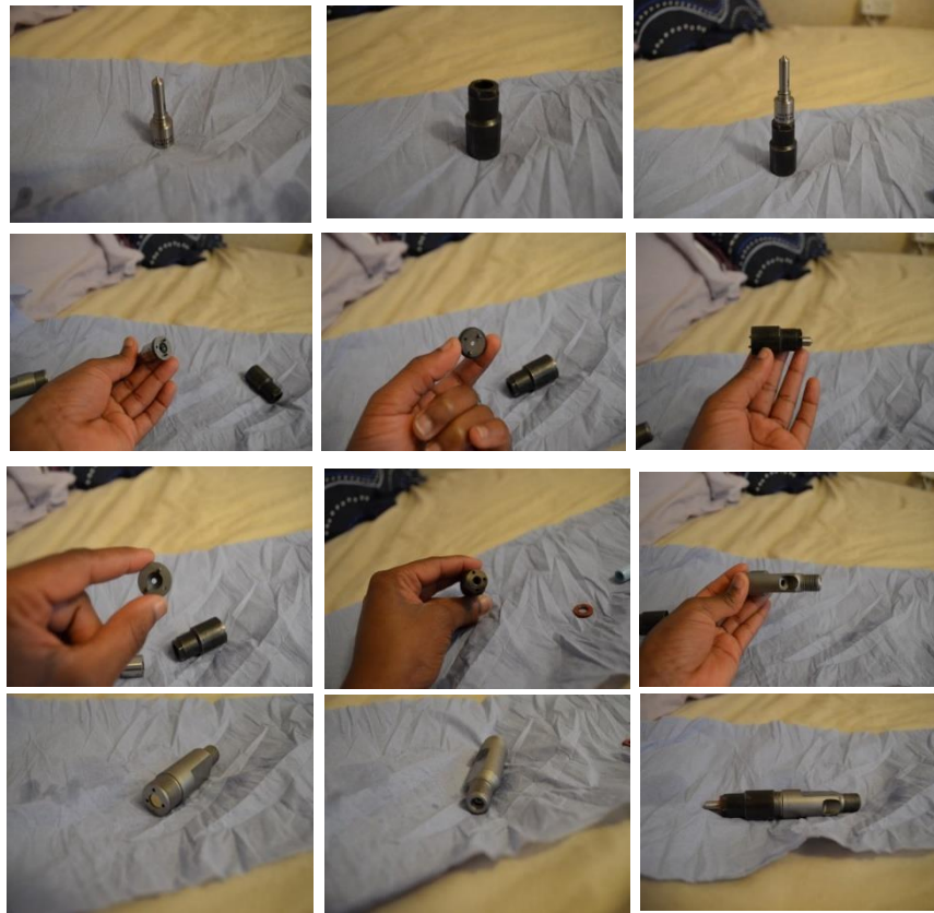
Figure B 2 - 2 Components of the needless 0.4 mm hole diameter HB X 6965489 single hole Cylindrical nozzle
