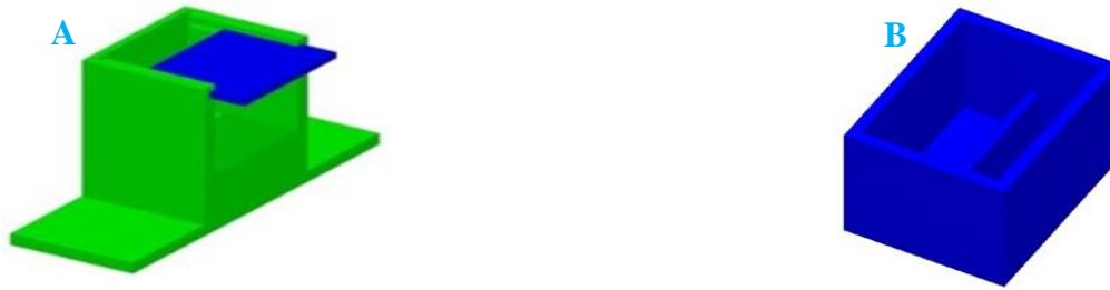
Figure 5.1: A) Custom made plastic holder, B) Custom made plastic mould for phantom's construction.
