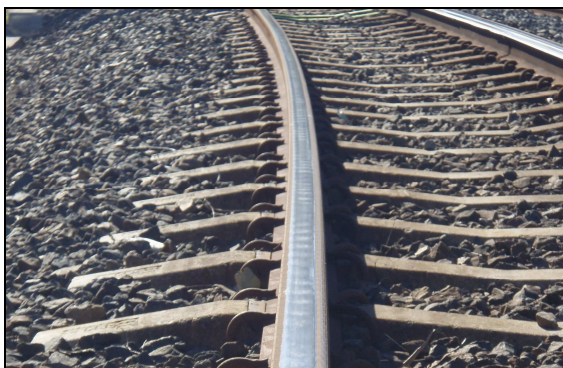
Figure 1. 9 month old corrugated rail profile
