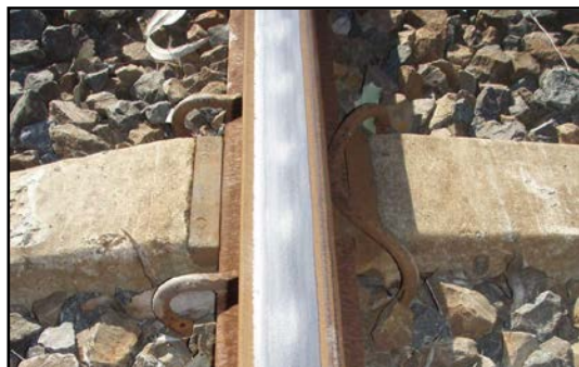
Figure 1 - 9-month-old corrugated rail profile
