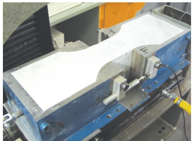
Figure 7. Fly ash specimen ready for uniaxial tensile test
