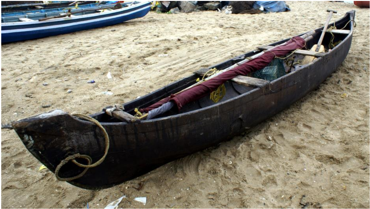
Fig. 1. Hūrī ready for use on the beach at Calicut, Kerala. This example used for fishing by a single fisherman, it is rigged for sailing as well as being propelled with a single paddle when leaving/returning to the beach. It is primarily a logboat hull, with some small areas of repair. A false frame is visible underneath the sail and adjacent to the central thwart in the photograph (Photo: J. Whitewright).
