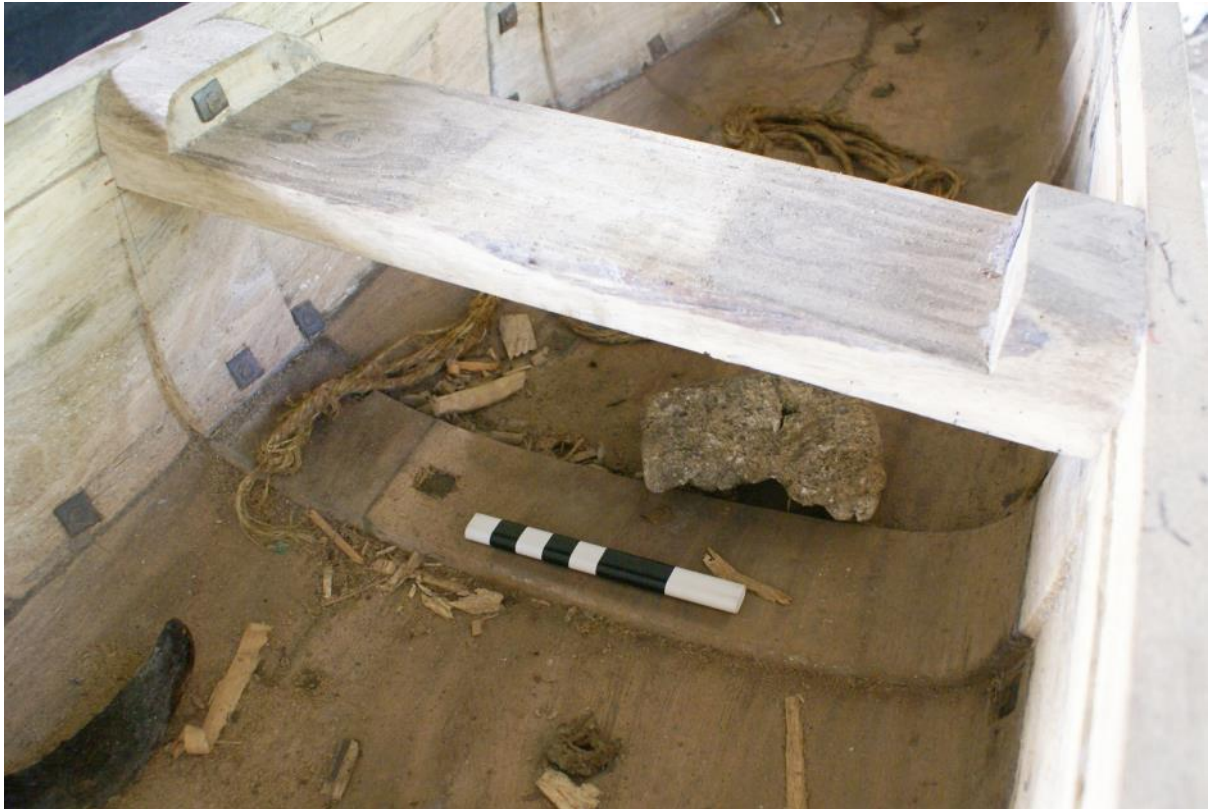
Fig.4. A false frame on the log-based plank-built hūrī illustrated in figure 5. The false frame occupies the log-base of the vessel, but also clearly extends across the additional shell-based planking that is used to form the shape of the vessel's hull. The iron rivets used to fasten these planks together are also visible. Scale = 20cm (Photo: J. Whitewright).
