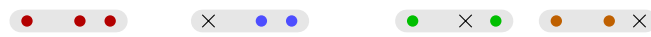
Figure 2.7: Thinned shift-invariant array of M = 9 , obtained by removing sensors from the virtual shift-invariant array of P = 4 sensors with M_0 = 3 sensors per subarray, given in Figure 2.5
