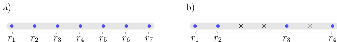
Figure 2.2: a) Uniform linear array of M = 7 sensors and b) thinned linear array of M = 4 sensors, obtained by removing sensors from a virtual uniform linear array of M_0 = 7 sensors
