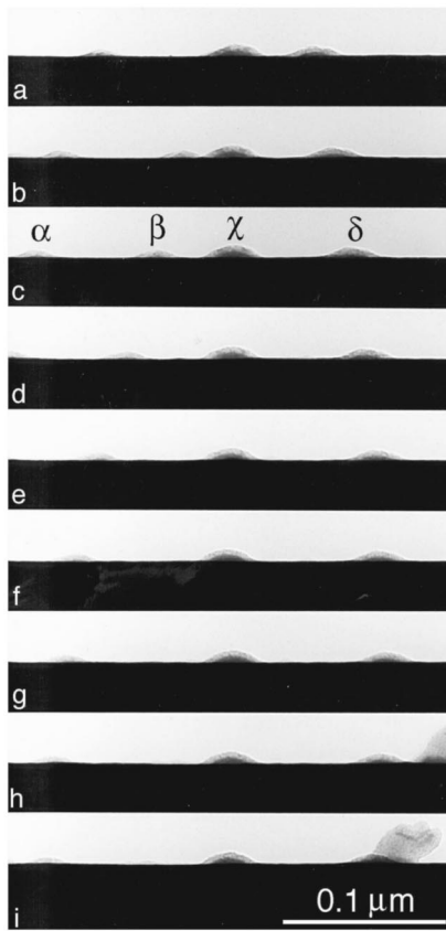
FIG. 2. A series of bright-field images obtained by tilting the TEM specimen along the [001] axis. The quantum dots \chi has been put into the center of the image to carry out a detailed analysis.
