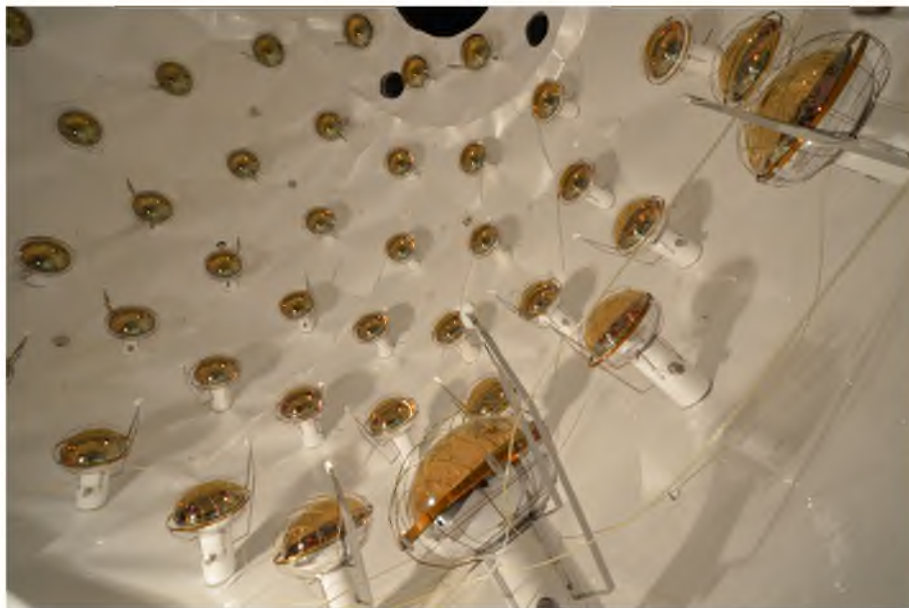
Figure 3. The Liquid Scintillator Veto. The picture shows the internal surface of the LSV, covered with Lumirror, with PMTs evenly distributed inside.
