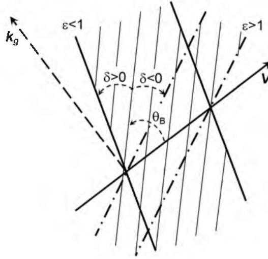
Fig. 2. Two possible orientations of the plate surface for a fixed angle  $\theta_B$ . The first one corresponds to  $\varepsilon < 1$ , the second one corresponds to  $\varepsilon > 1$ .
