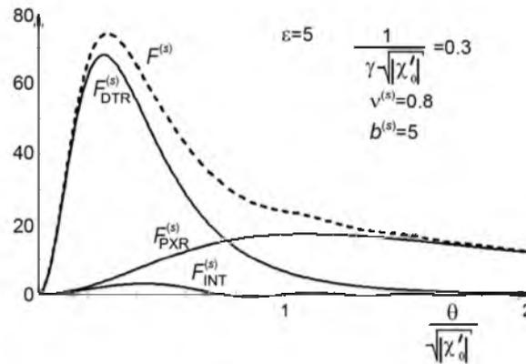
Fig. 9. Angular density of radiation in an asymmetrical case for higher electron energy than in Fig. 8.
