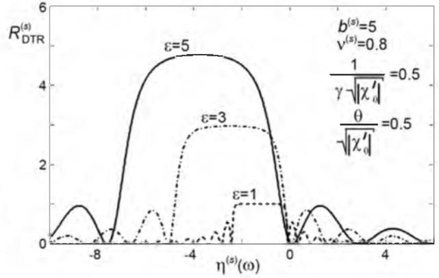
Fig. 6. Effect of asymmetry on the DTR spectrum.
