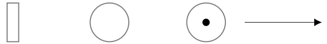
Figure 1: Basic PN components presented from left to right: 1) transition, 2) place, 3) marked place, 4) arc.
