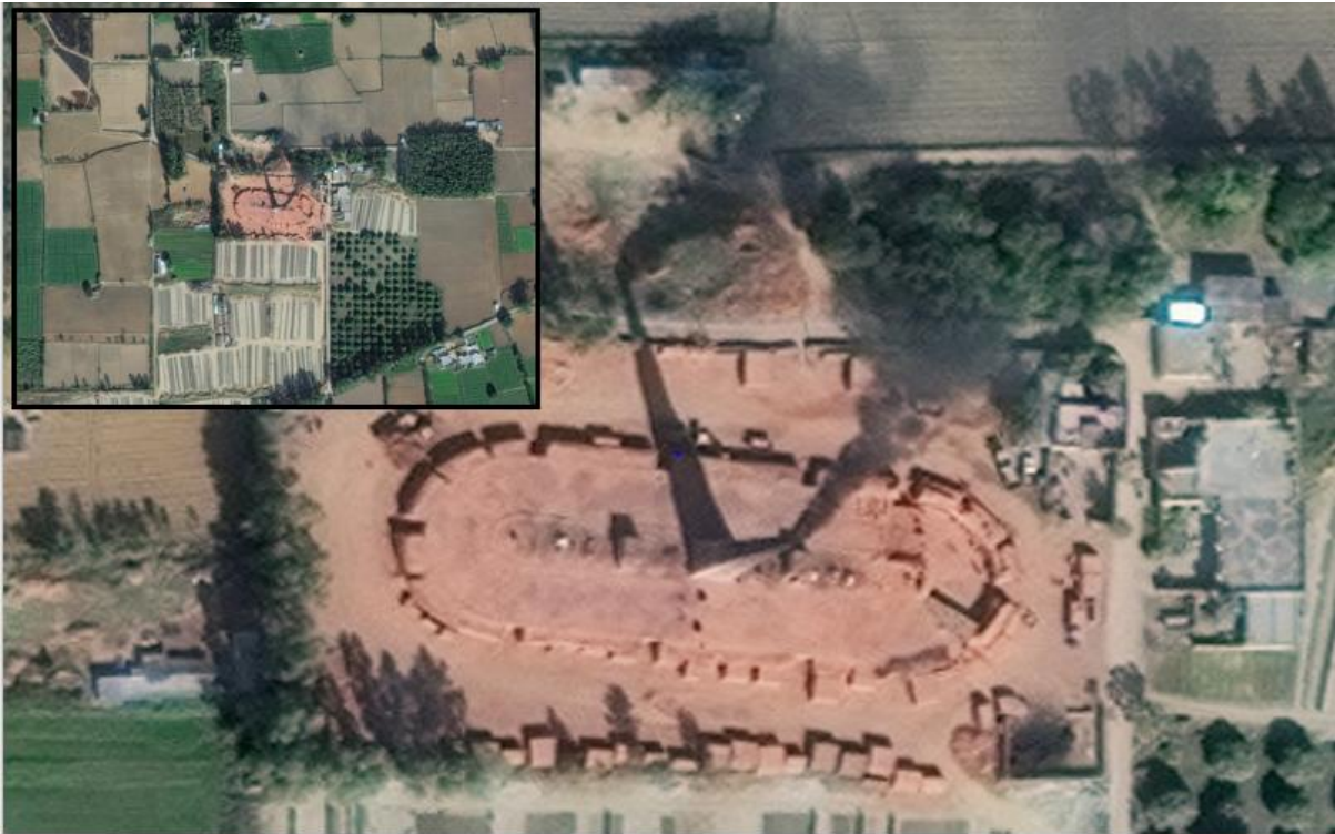
Figure 7: An example of a Fixed Chimney Bull's Trench brick kiln @31.5385546, 75.9813821 – note the emissions from the chimney stack. From Digital Globe's WorldView-2 satellite system; pan-sharpened natural colour at 50cm resolution; captured in November 2015.
