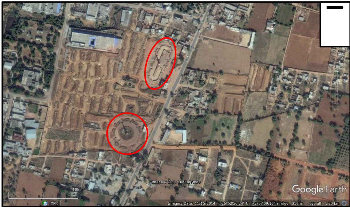
Figure 2: An image featuring two brick kilns. One is a traditional Bull's Trench Kiln (BTK) and the other is a circular kiln. Surrounding these kilns is a number of clay fields that are used in the production of the bricks themselves before the firing of the bricks in the kilns. These fields are commonly found close to the kilns although sometimes they are not directly adjacent to the kilns.
