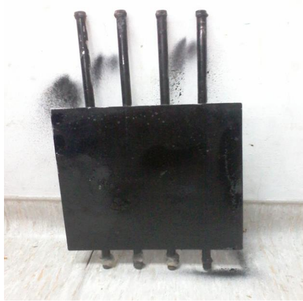
Figure 6-5: Solar thermal collector after black coating
