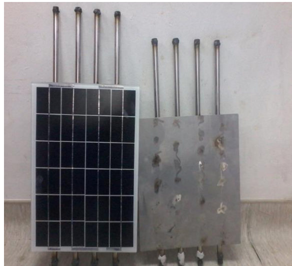
Figure 6-3: Snapshot of PV/thermal and thermal collector.
