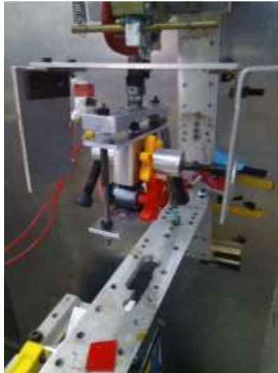
Fig 6. 35 Generator gears were changed to one that are taken from toys.
