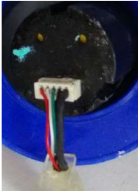
Fig 3.5 Connector input to the encoder.
