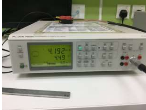
Fig A. 2 The RCL meter, along with the measurements
