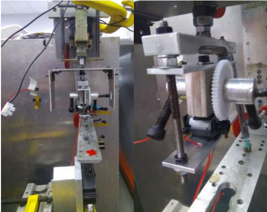
Fig 6. 32 the photograph on the left shows the generator attached to the pendulum, on the right shows the view of how the motor is held by a plate that is attached to the pendulum support.
