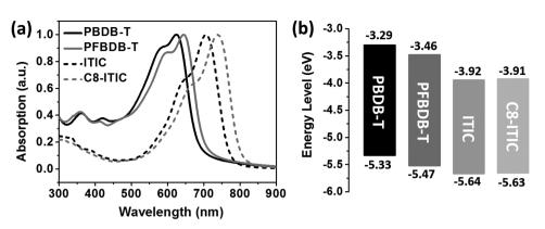
Figure 1. a) Thin film UV-vis absorption spectrum and b) energy levels (calculated from CV) of PBDB-T, PFBDB-T, ITIC and C8-ITIC in drop-cast films.
