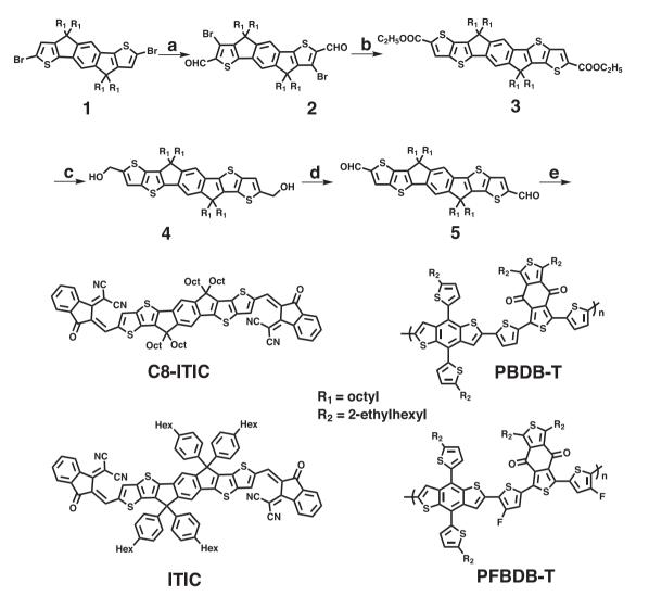
**Scheme 1.** The synthetic route to C8-ITIC and the structures of ITIC, PBDB-T, and PFBDB-T. a) Lithium diisopropylamide (LDA)/dimethylformamide (DMF)/76%, b) ethyl mercaptoacetate/K<sub>2</sub>CO<sub>3</sub>/DMF/69%, c) lithium aluminum hydride (LAH)/tetrahydrofuran (THF)/90%, d) Dess–Martin periodinate/THF/85%, e) (3-dihydro-1H-inden-1-ylidene)malononitrile/pyridine/CHCl<sub>3</sub>/82%.
