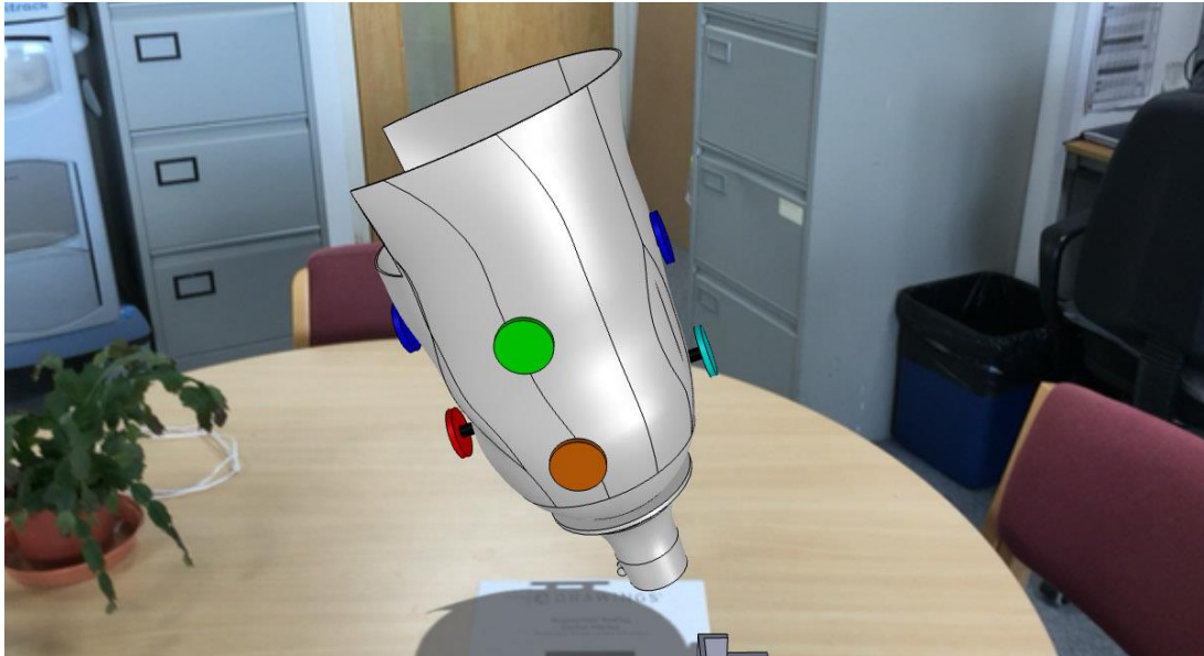
Figure 96 - Augmented reality application prototyped in this project. Orientation and load values can be visualised on a realistic socket model
