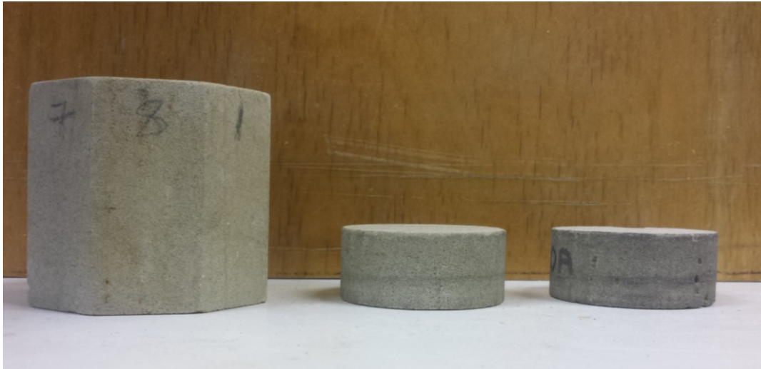
Figure 1. Octagonal, blank and 90° fractured rock samples respectively (from left to right).
