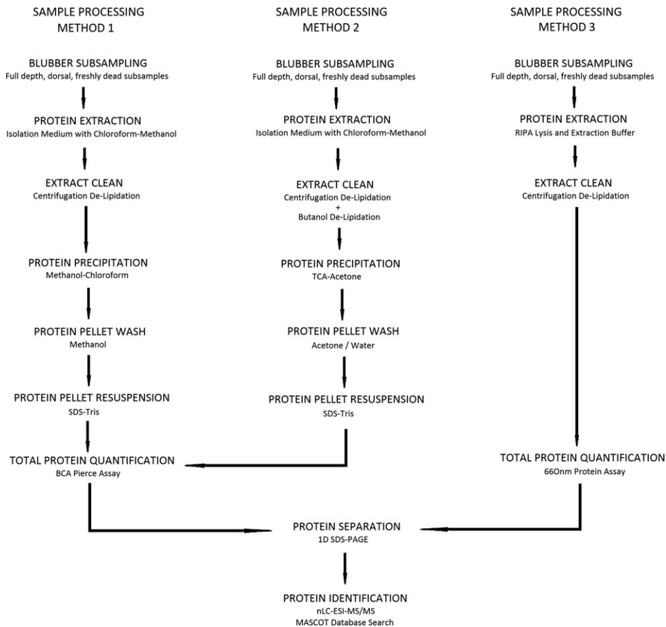
Figure 1: Workflow showing the sample processing methods for protein extraction, quantification, separation and identification. Sample processing Methods 1 and 2 involve various extract cleaning, protein precipitation and protein pellet wash stages. Sample processing Method 3 involves fewer processing stages. The extracts using all three methods were used for downstream analyses; protein quantification, separation and identification.
