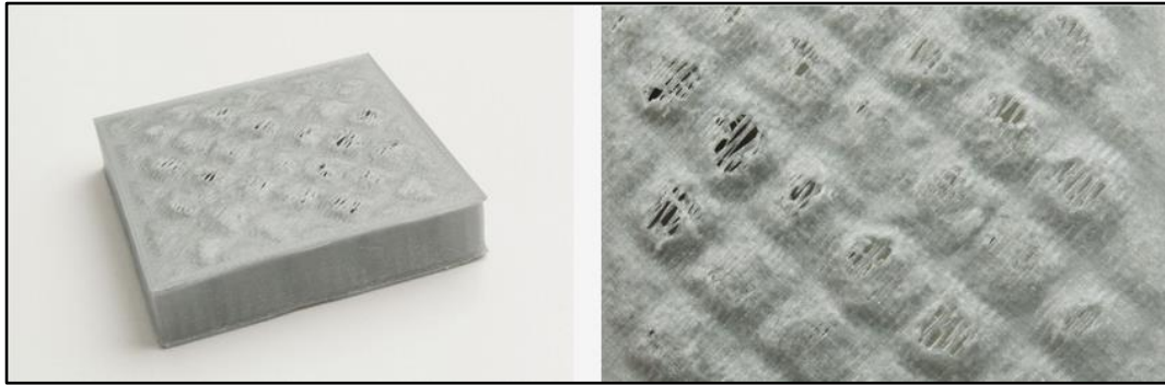
Figure 22: Effect of Inadequate Cooling in a 3D Print
