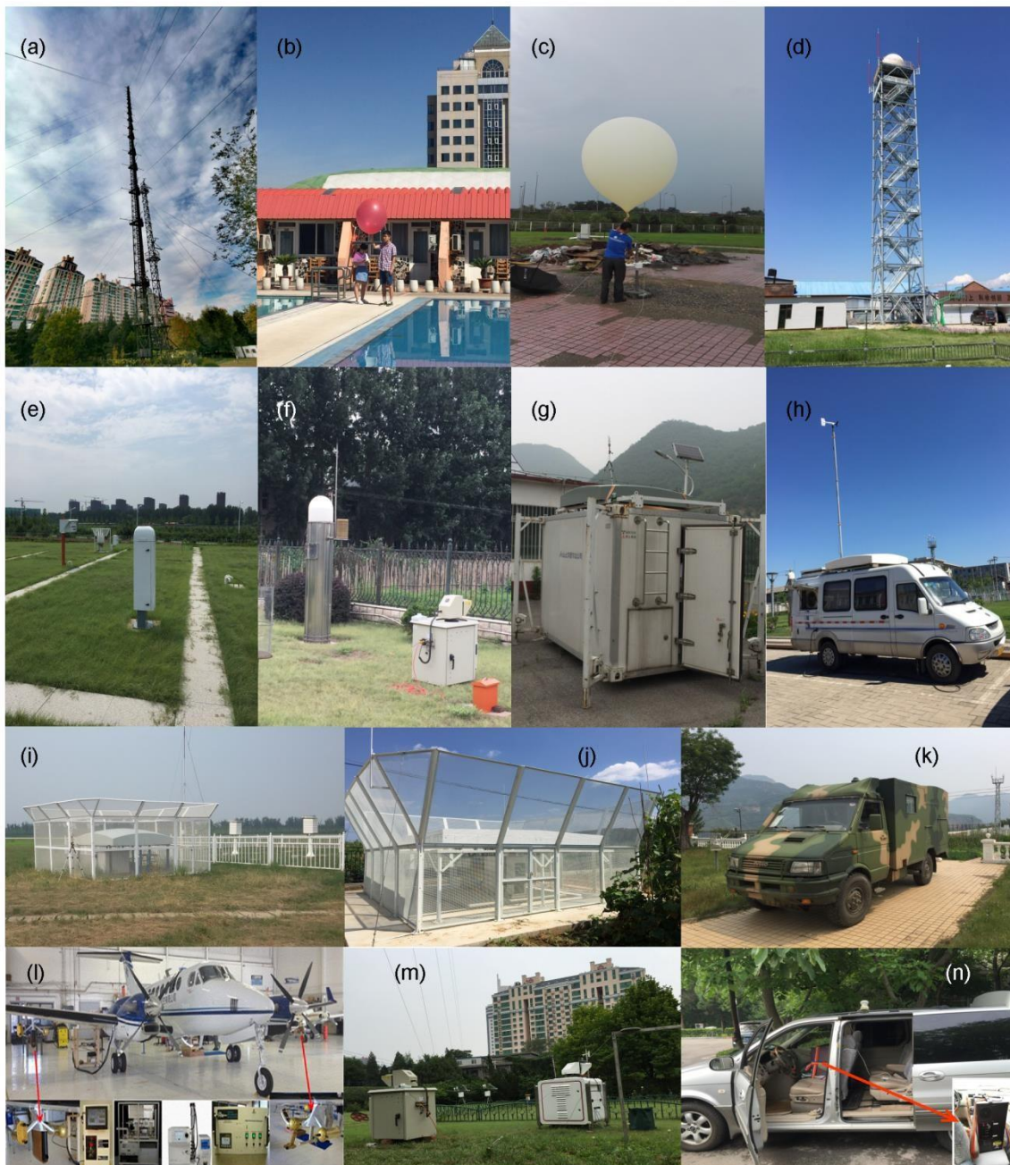
Fig. 2. Photographs of some SURF instrumentation (a) 325-m tower at IAP, (b) small balloon radiosonde at IUM, (c) GPS radiosonde at NAN, (d) X-band radar at SHU, (e) ceilometer at LIA, (f) Mini-MPL at DAX, (g) wind profiler at SID, (h) mobile wind profiler at CHA, (i) wind profiler at SHA, (j) wind profiler at YAN, (k) wind profiler at GUC, (l) King Air airplane, (m) Doppler lidar and Mini-MPL at IAP, and (n) mobile MPL, where three letter abbreviations are defined in Supplement A.
