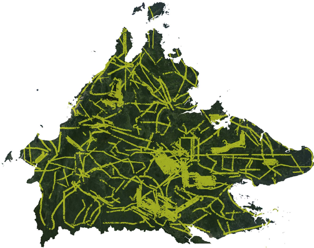
Fig. A2. Distribution of data collection flightlines from the Carnegie Airborne Observatory sampling of Sabah. Each line is 1.5–3.0 km wide (swath). Areas of particularly concentrated mapping coincide with landscapes containing field calibration plots.
