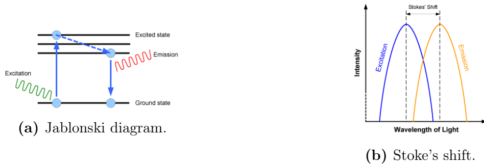
Figure 1.3 Fluorescence: Excitation and de-excitation of a fluorescent molecule (Jablonski diagram) and Stokes’ shift between the absorption and emission spectra.
