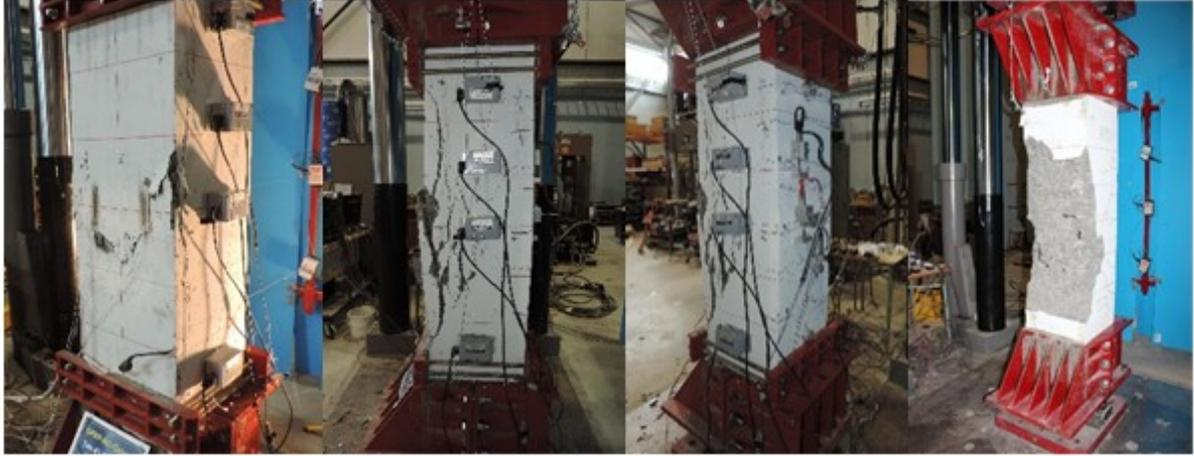
Figure 9. Crack appearance and failure mode of columns tested under low eccentricity ( $e/h_o = 20\%$ ; G1)
