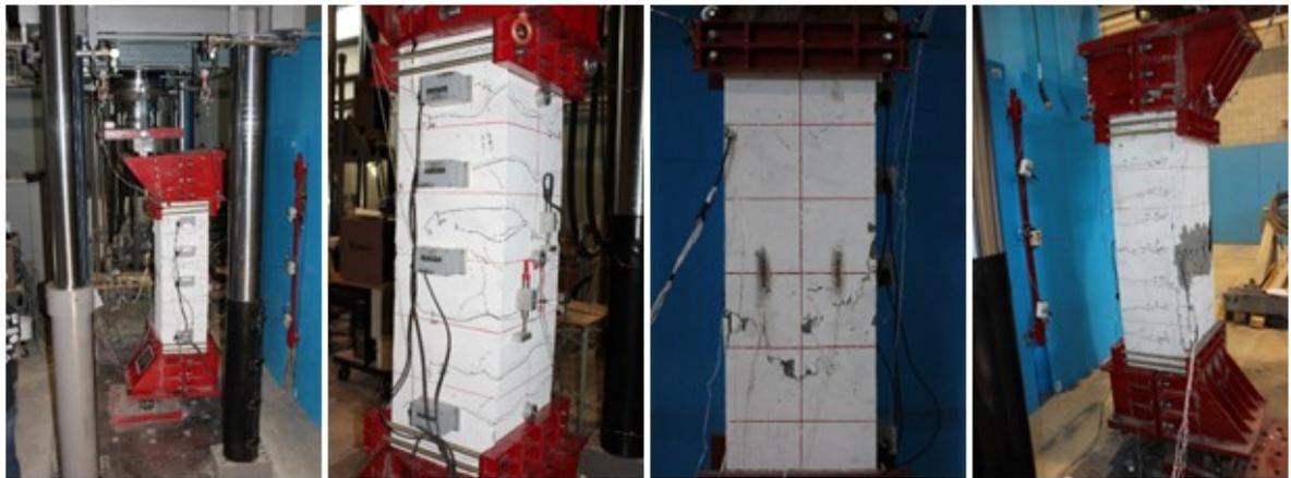
Figure 11. Crack appearance and failure mode of columns tested under large eccentricity ( $e/h_o = 80\%$ ; G2)
