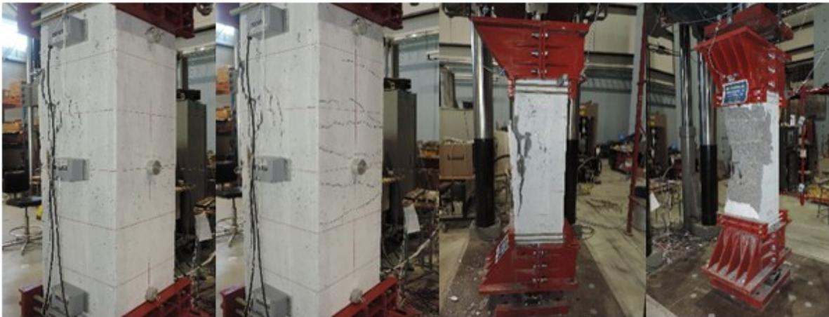
Figure 8. Crack appearance and failure mode of columns tested under low eccentricity ( $e/h_o = 10\%$ ; G1)
