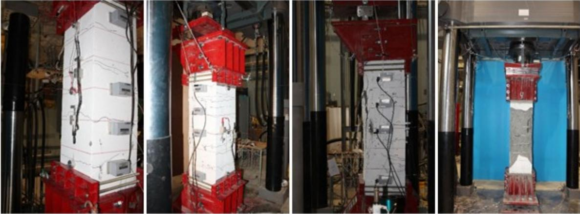
Figure 10. Crack appearance and failure mode of columns tested under moderate eccentricity ( $e/h_o = 40\%$ ; G2)
