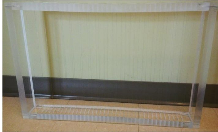
Figure 5.2: A sample frame designed to allow various folding ratios of drapes
