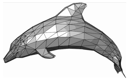
Figure 2.5: Triangulated Surface Representation [28]
