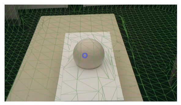
Figure 2.10: Spatial Understanding Mesh Overlaying an Object in the HoloLens view
