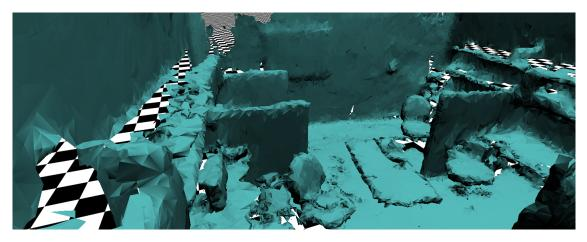
Figure 2.6: 3D Mesh of an Office Space as Scanned by the Microsoft HoloLens
