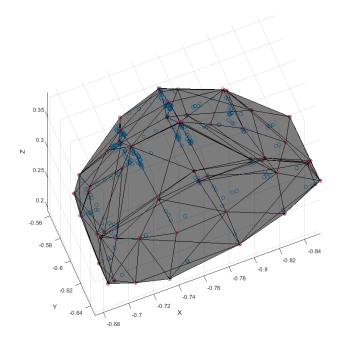
Figure 4.4: Convex Hull Created for the Filtered Point Cloud Using MATLAB (X, Y and Z are 3D Coordinates Representative of Distance in Meters)
