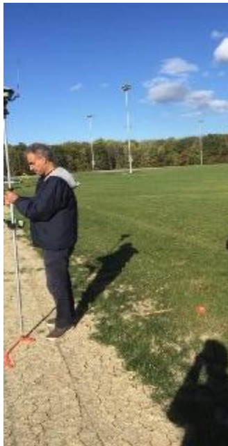
Figure 5.13: (a) Ground truth measurement using RTK system, (b) schematic of a simulated polygon on the ground.
