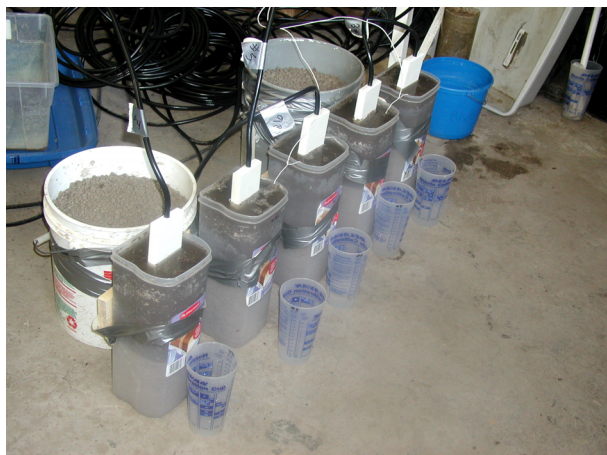
Figure 2. Performing soil TDR experiments in the laboratory.
