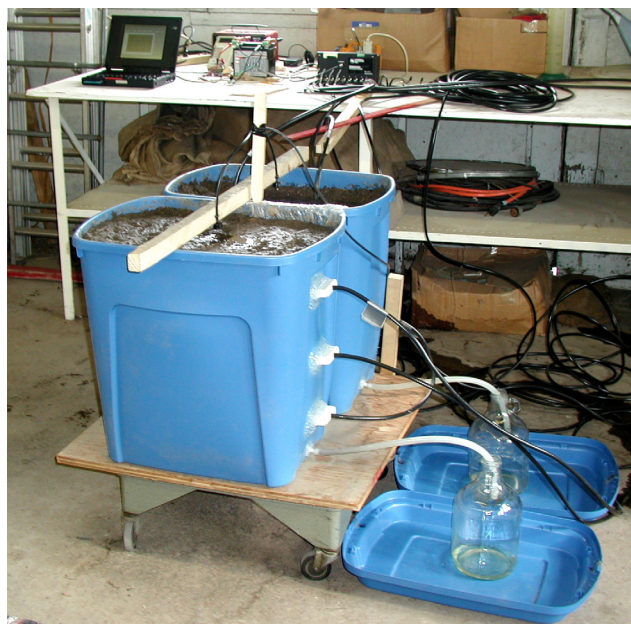
Figure 3. Laboratory lysimeter setup.
