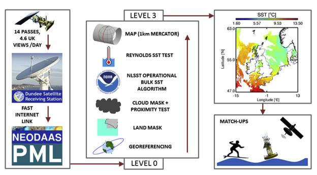
Fig. 3. Schematic diagram of the NEODAAS system for producing the operational AVHRR SST products used in the study.
