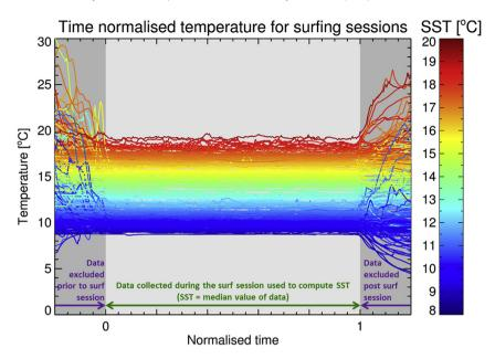
Fig. A3. A superposition of all temperature data acquired by the surfer during the study period, normalised such that the start (0) and end (1) of the surfs are at the same point on the x-axis for each session. Data in dark grey were excluded and light grey included. The data in light grey were used to compute SST by taking the median of this data.
