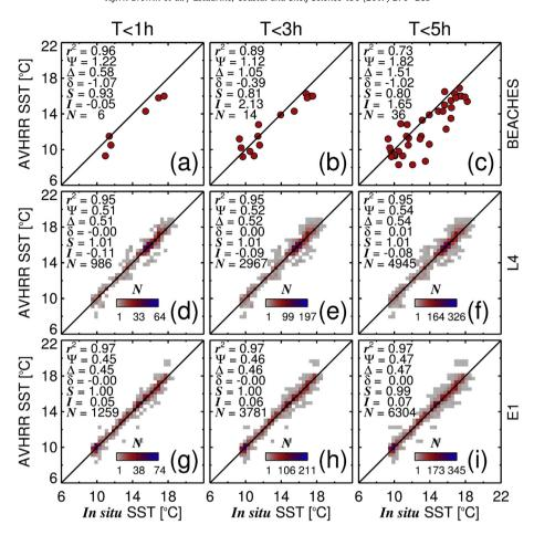
**Fig. 7.** Scatter plots of Level 3 AVHRR satellite passes and *in situ* sea surface temperature (SST) data for an absolute time difference (T) of <1 h, <3 h and <5 h, at the coastline (a–c), at L4 (d–f) and at E1 (g–i).  $r^2$  is the coefficient of determination, Ψ the root mean square error, δ the bias, Δ the centre-pattern (or unbiased) root mean square error, S the slope and I the intercept of a linear regression, and N the number of samples.
