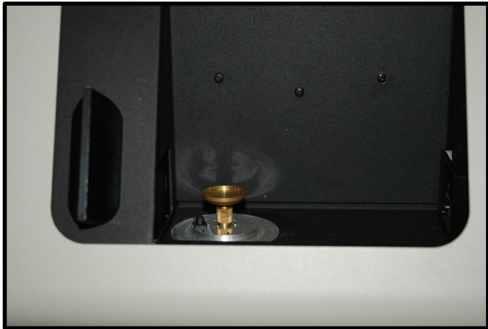
Figure 9-10. The circular platform stage fixed inside the Skyscan 1174 micro-CT scanner
