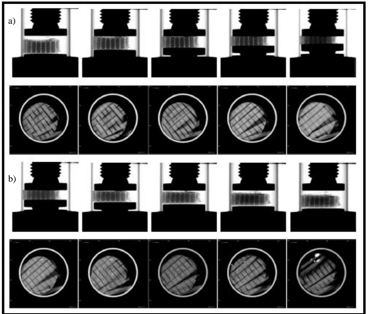
Figure 9-23. Micro-CT scans of the compression and release of the dry fibre 3Tex 3D woven fabric. a) the compression of the fabric specimen shown with cross section scans along the y axis and reconstructed images of a single point along the z axis b) the release of the fabric specimen shown with cross section scans along the y axis and reconstructed images of a single point along the z axis
