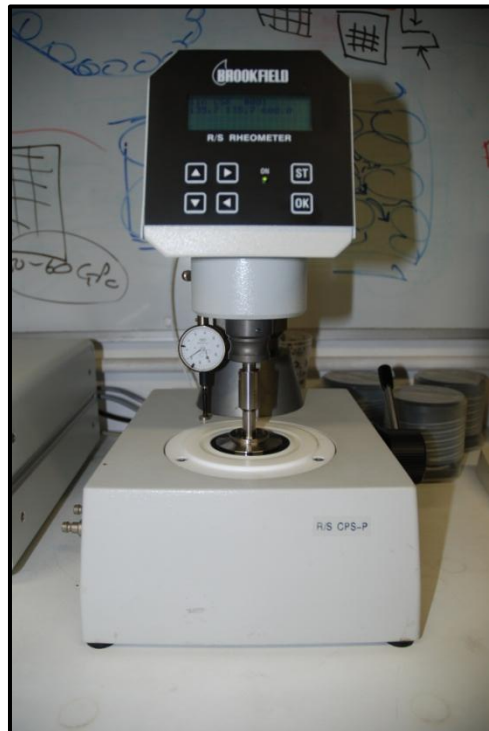
Figure 9-2. The RS Brookfield Rheometer employed to measure the dynamic viscosity of the experimental liquid.
