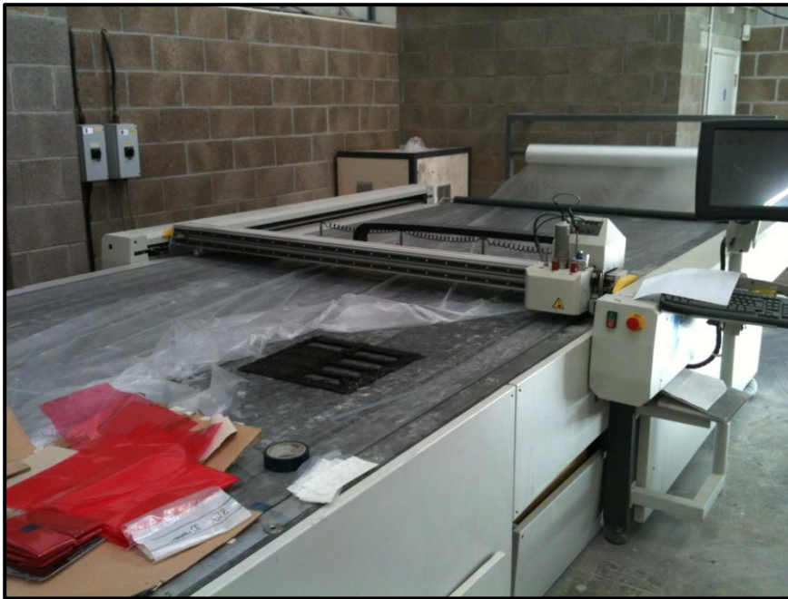
Figure 3-22. The CNC ply cutter employed to cut the tufted preform samples at Pipex ltd [100]
