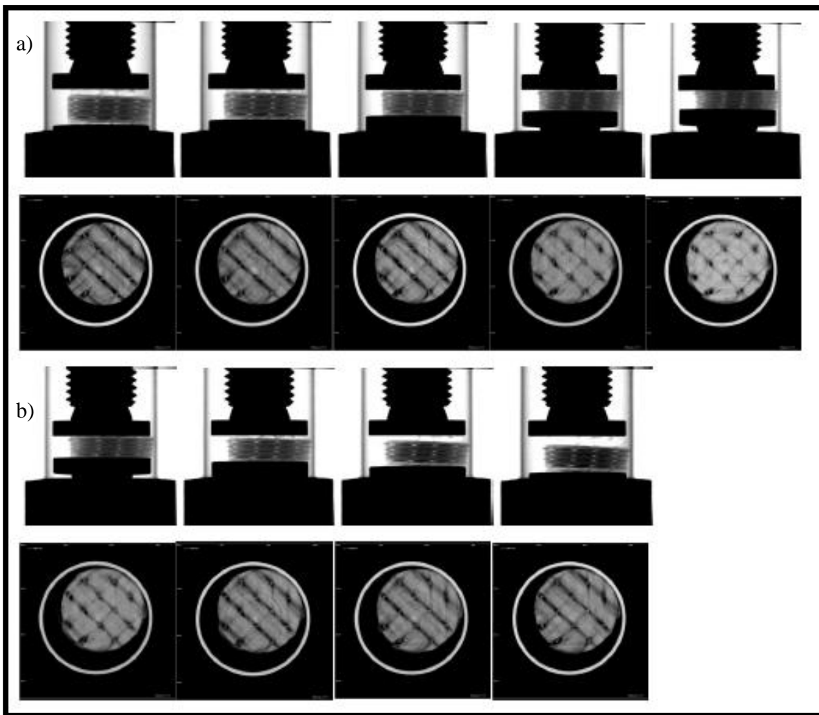
Figure 9-24. Micro-CT scans of the compression and release of the dry fibre Saertex quasi NCF 4x4 tufted fabric. a) the compression of the fabric specimen shown with cross section scans along the y axis and reconstructed images of a single point along the z axis b) the release of the fabric specimen shown with cross section scans along the y axis and reconstructed images of a single point along the z axis
