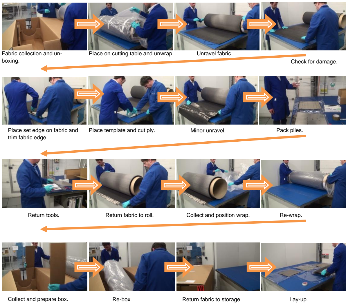
Figure 3-8. Visual summary of the fabric cutting and lay-up sub process
