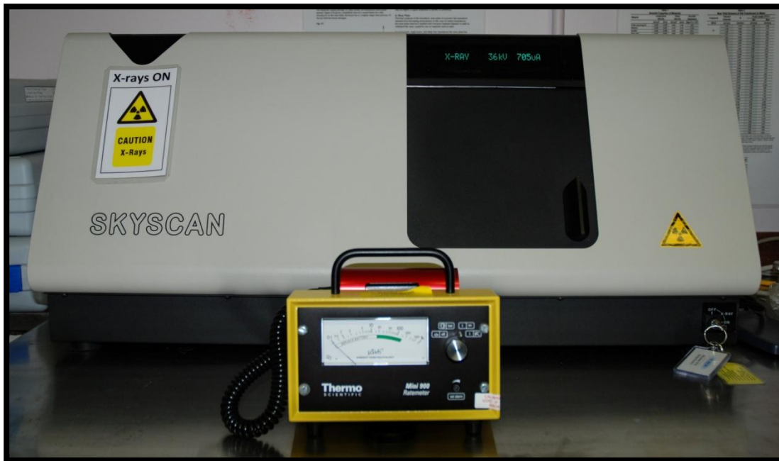
Figure 9-8. The Skyscan 1174 micro-CT scanner and the Thermo Fisher Scientific Mini 900 rate meter
