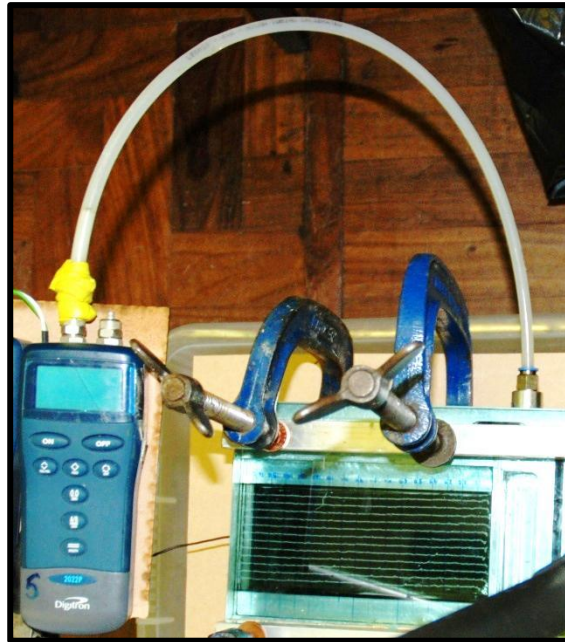
Figure 9-1. Differential pressure gauge arrangement
