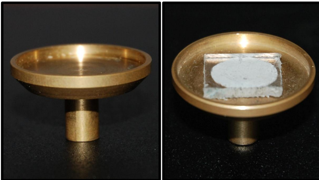
Figure 9-9. The circular platform stage for the Skyscan 1174 micro-CT scanner, with and without spacer
