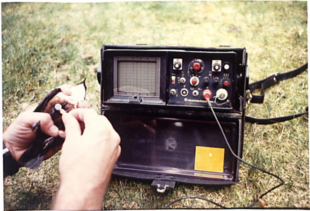
Fig. 8.1a Field application of ultrasonic flaw detector for measurement pectoralis muscle thickness in a Dipper.
