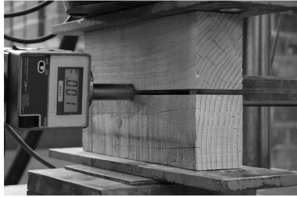
Fig. 5 Friction test on dynamic test specimens
