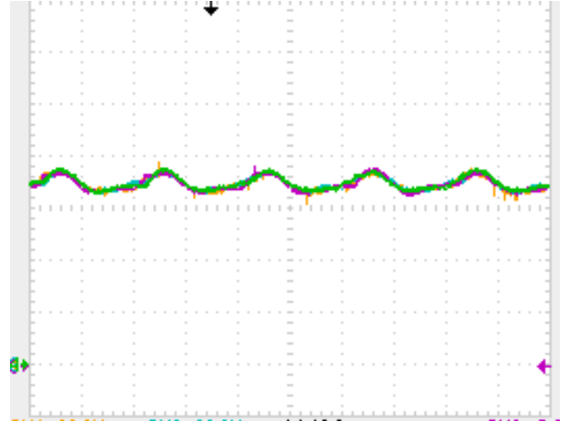
(e) per arm cell capacitor voltages (10ms/div and 20V/div)
