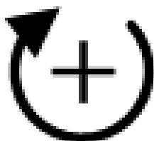
Figure 6.6 A Reinforcing Loop (CLD)
