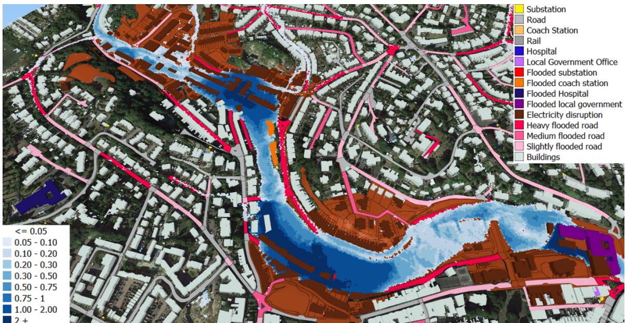
Fig. 4. 3D view of Clis, roads and buildings near the coach station in Torquay under 1 in 100 year return pluvial flood event
