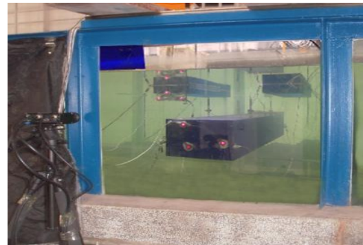
Fig. 4 Tunnel and twin-barge configuration: (a) mooring line coordinates (b) 6D-Ums configuration
