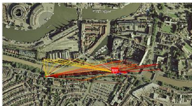
Fig. 1. Point to point ray-tracing and the resulting rays between BS and OBU.
