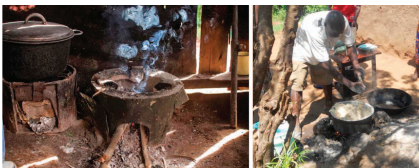
Figure 2. Kuni M'Bili ICS stove (left) and three stone open fire (right), Nyeri County, 2014.
