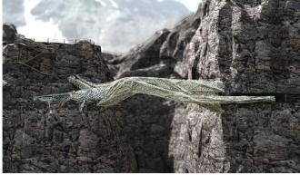
Supporting new methods of architectural design and production using autonomous robotics, multi-agent control, construction simulation and environmental awareness. Left: Adaptive additive manufacturing in response to live scan data. Top-right: Aerial Additive Building Manufacturing (ABM) multi-agent construction simulation. Bottom-right: Aerial ABM bridge design
