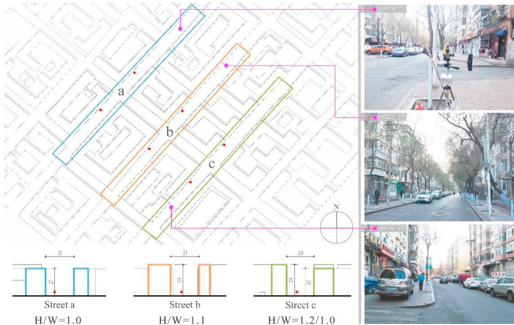
Fig. 2. Street measuring point arrangement and street real scene
