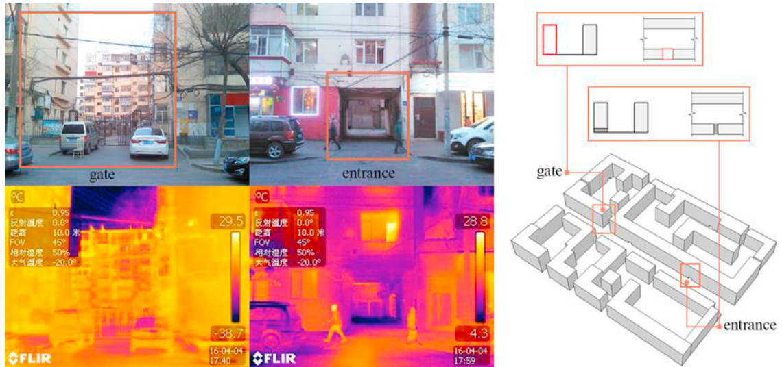
Fig. 6. Infrared images the classifications of facade openings
