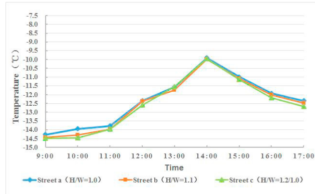
Fig. 4. Air temperature change curve of different aspect ratio streets
