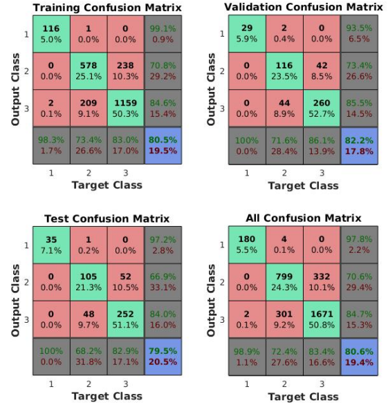
Fig. 2. Result of classification of oil, water and gas dataset. The first three diagonal cells show the number and percentage of correct classifications by the trained network. For example, in the test confusion matrix (bottom right matrix in Fig. 2) 35 water samples are correctly classified as water (class 1) which corresponds to 7.1% of all 493 samples. Similarly, 105 cases are correctly classified as gas and this corresponds to 21.3% of all samples and 51.1% are correctly classified as oil and this corresponds to 51.1% of all samples.
